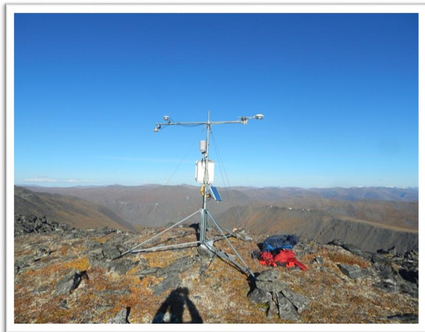
Meteorological station in the southwest Yukon at ~2200 m asl from June 2012. Photo by Scott Williamson.
